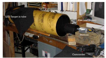
aimed at a dark field containing a target LED of adjustable brightness. The Mintron video output feeds through a so-called Kiwi OSD (On Screen Display). The Kiwi is a device that uses a GPS sensor to detect the UTC time to an accuracy of about 1us. This time is used to calculate the beginning and end of each video field, and is electronically pasted onto each video field in human readable form. The time stamped video is then sent to a camcorder.
