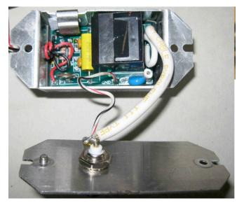
layers of electrical tape (not shown) around the center BNC contact. Using 6-32 screws in place of the rivets, reassemble the unit (replacing the heat sink clip and tape as they were).
