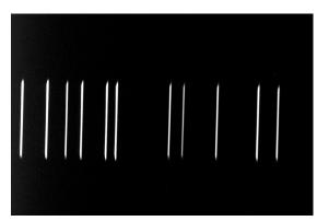
The slit is also not quite vertical to the grating lines, thus causing the line tilts. The band is also very slightly below the center of the frame, which shows that the grating tilt is not perfect. For most stellar spectroscopy, this degree of imperfection is easy to handle in the image processing.
